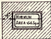
Brick with Flue Lining.
