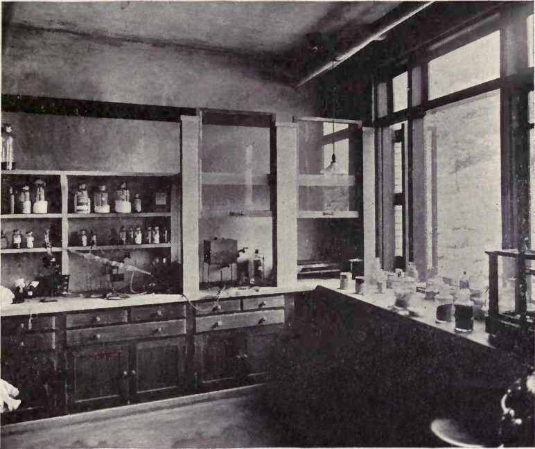
Fig. 264.—Alberene stone hood, Melon Institute, Pittsburg, Pennsylvania. By courtesy of the Alberene Stone Company.
