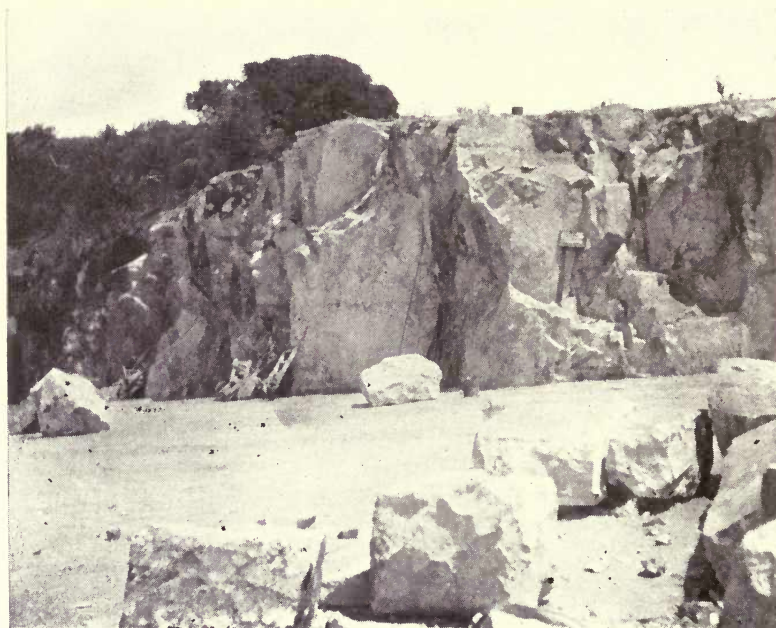
Fig. 123.—Quarry in volcanic tuff, Los Berros, San Luis Obispo County, California. The material is used for building purposes. Photo. by T. C. Hopkins.
