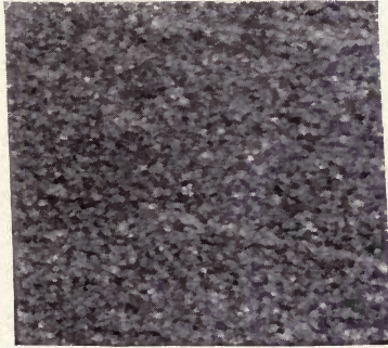
Fig. 127.—Polished slab of quartzose marble from quarry of Huntington and Clough, Washington, Vermont. Photo. by C. H. Richardson.
