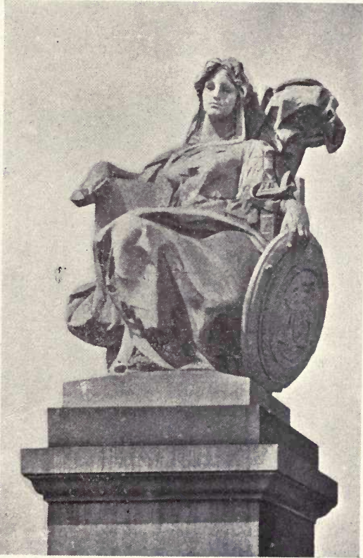
Fig. 37.—Carving from the light gray, fine textured, biotite-muscovite granite from the Stinchfield quarry, Hallowell, Maine, showing adaptation to delicate sculpture. By courtesy of the U. S. Geological Survey.
