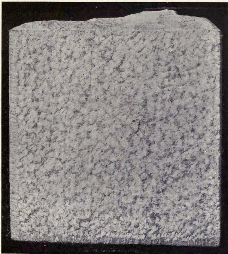
Fig. 224.—Block of Potsdam sandstone, Potsdam, New York, showing tooled surface. Photo. by C. H. Richardson.
