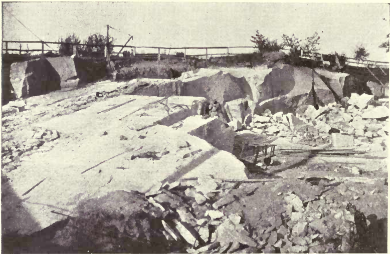
Fig. 71.—Granite quarry, Newport, Vermont, showing thickness and curvature of sheets. Photo. by C. H. Richardson.
