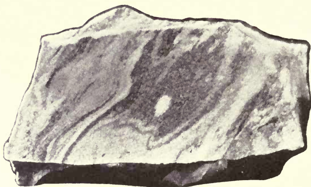
Fig. 179.—Polished block of Wait's River marble, Wait's River, Vermont, from H. C. Richardson quarry. The sample was polished in 1893 and photographed in 1916. Photo. by C. H. Richardson.
