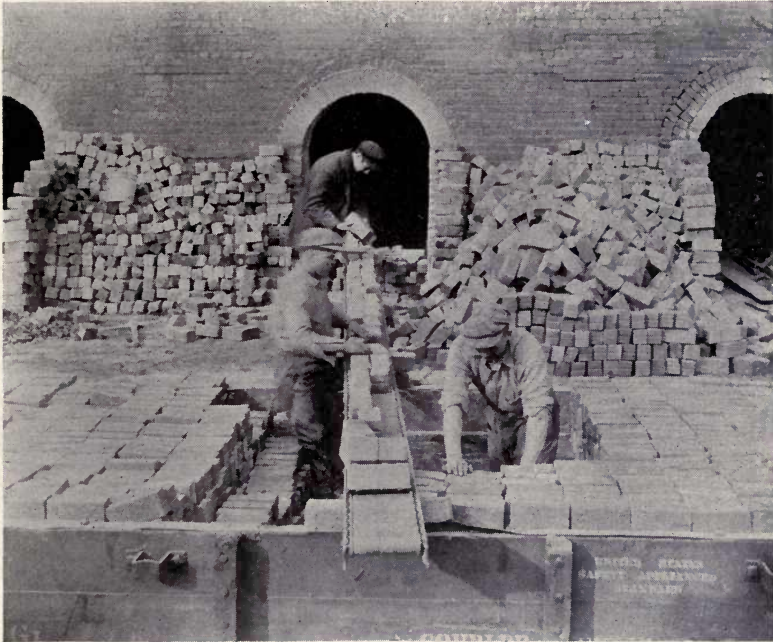
Fig. 294.—Manufactured brick coming out of the kiln on a gravity carrier. An inspector is standing next to the door rejecting the brick not going into the class of those being loaded into the car for shipment. By courtesy of the National Paving Brick Manufacturers Association.
