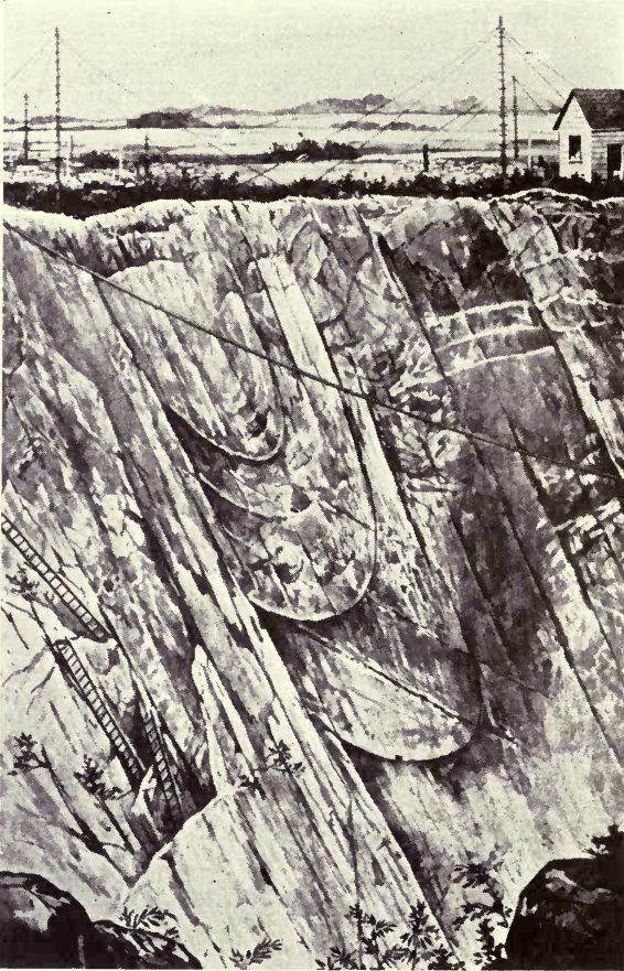
Fig. 250.—Rising and Nelson slate quarry, Pawlet, Vermont, showing syncline in the seagreen slate. Depth 100 ft. By courtesy of the U. S. Geological Survey.
