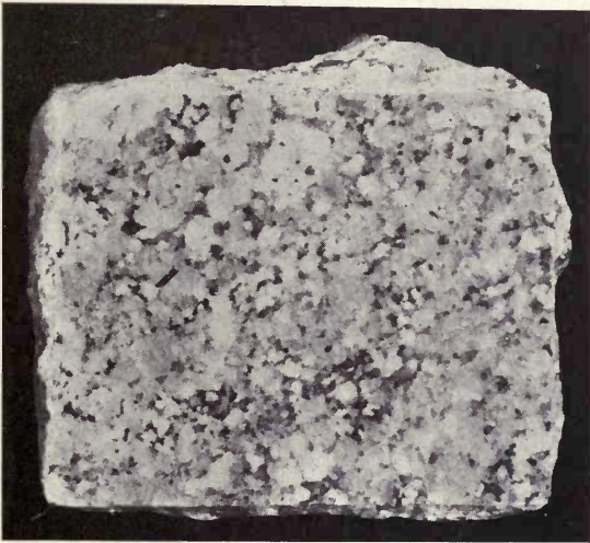
Fig. 33.—Polished slab of Stony Creek granite, Stony Creek, Connecticut. Photo. by C. H. Richardson.
