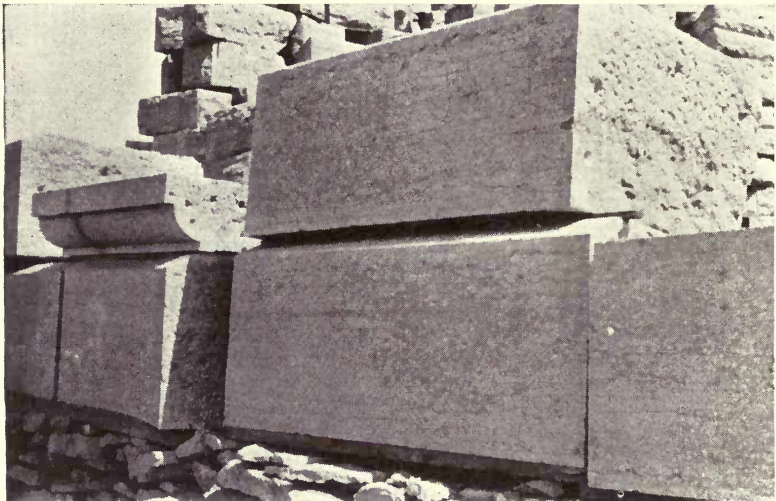
Fig. 215.—Blocks of gray sandstone, Cobleskill, New York, designed for constructional work in New York City. Photo. by C. H. Richardson.
