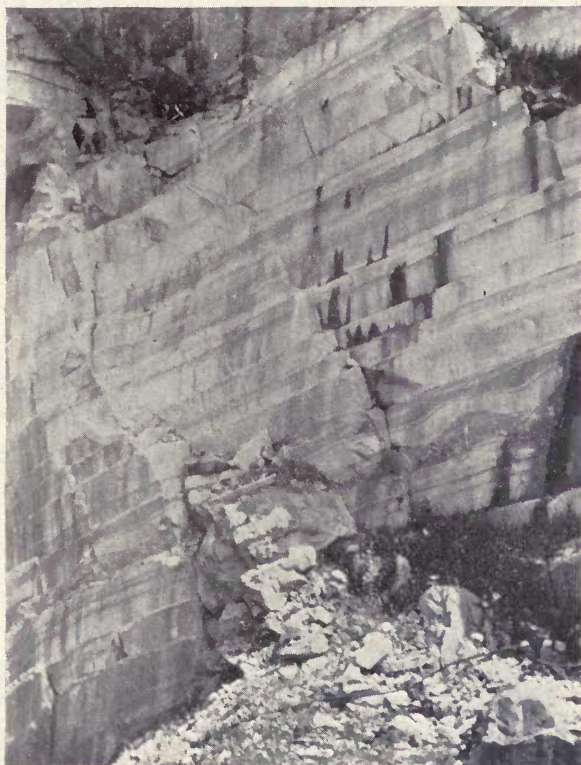
Fig. 161.—Interior view of marble quarry, West Rutland, Vermont, showing dip of the marble benches. Photo. by C. H. Richardson.
