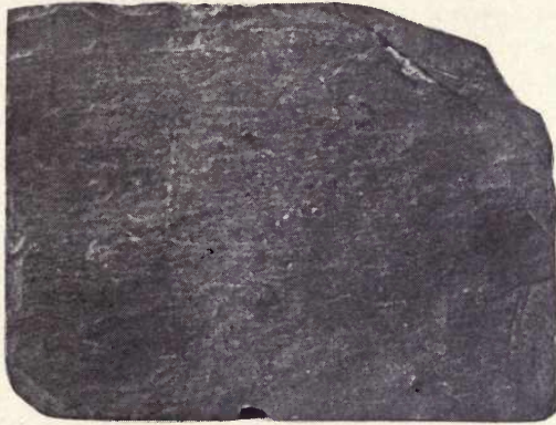
Fig. 251.—Slab of purplish black slate, Castleton, Vermont, showing perfect cleavage. Photo. by C. H. Richardson.
