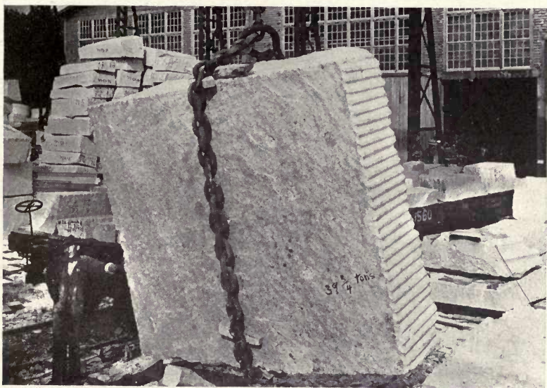
Fig. 117.—Method of chaining a large block of Bethel white granite. By courtesy of the Woodbury Granite Company.
