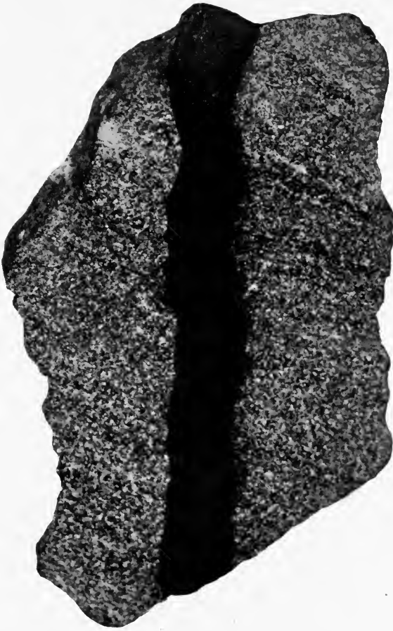
PLATE I. — A small fine-grained dike of dark diabase cutting a lighter-colored syenite. These dikes may be very narrow, or many feet in width.
