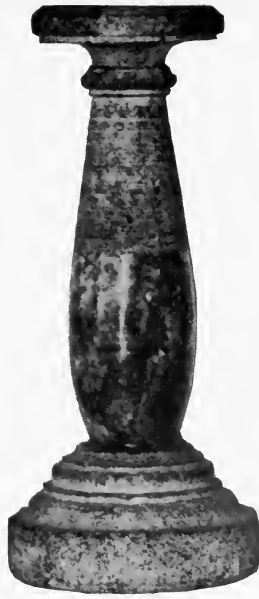
PLATE VIII, Fig. 1. — Gray marble, Gouverneur, N. Y., showing contrast between tooled and polished surface.
