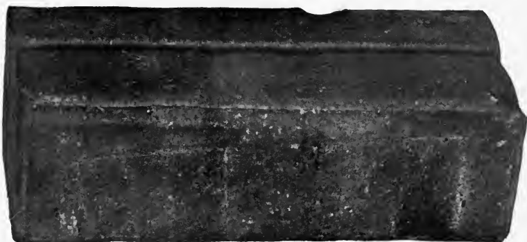
PLATE XLIX, Fig. 2. — Repressed brick. The rounded edges and corners as well as the grooves were produced in the repressing.
