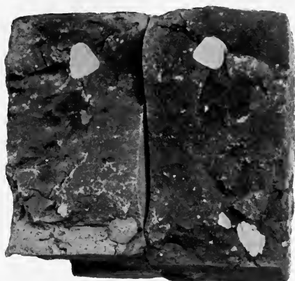
PLATE XLIX, Fig. 1.—Common red soft-mud brick which has been split by air slaking of calcined lime pebbles; the two white spots are the pebbles.
