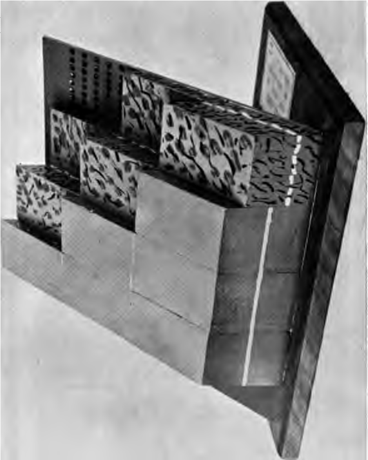
FIG. 14.—Model illustrating block caving mining sequence.
