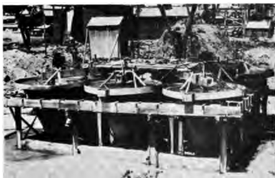
FIG. 15.—A battery of eight steel desliming cones.
