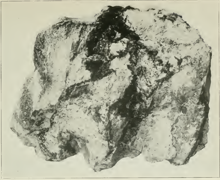
PLATE IV B. CRYSTALLINE WOLFRAMITE IN CAVITIES AND SEAMS OF RHYOLITE PORPHYRY, HENSAULT CLAIM, NEAR LEAD, S. D.
