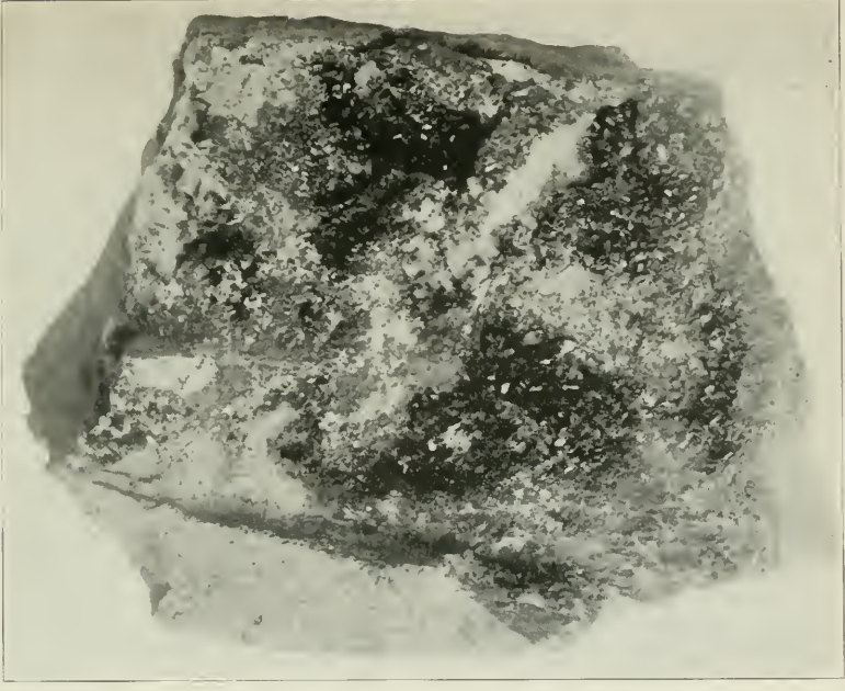
PLATE III B. WEDGE SHAPED CRYSTALS OF WOLFRAMITE GROWN IN OPEN CAVITIES. HOMESTAKE MINE, LEAD, S. D.
