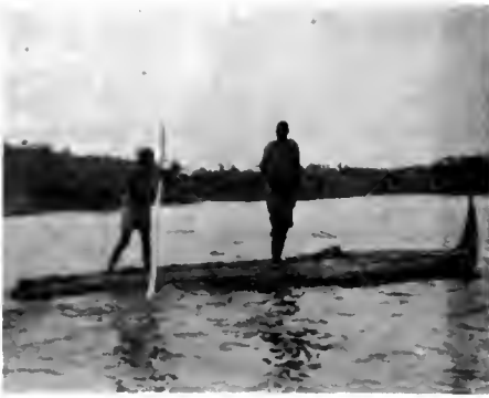
MYSTERY: WHY DOESN'T IT CAPSIZE? Canoe of papyrus reeds, made by the Buduma tribe, Lake Chad, northern Nigeria.
