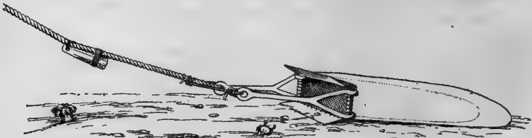
DREDGE FOR USE IN SHALLOW WATER.
