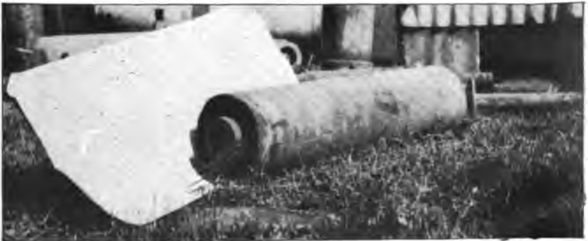
B. CYLINDER ON WHICH CARBON BLACK IS DEPOSITED IN ROLLER SYSTEM.
