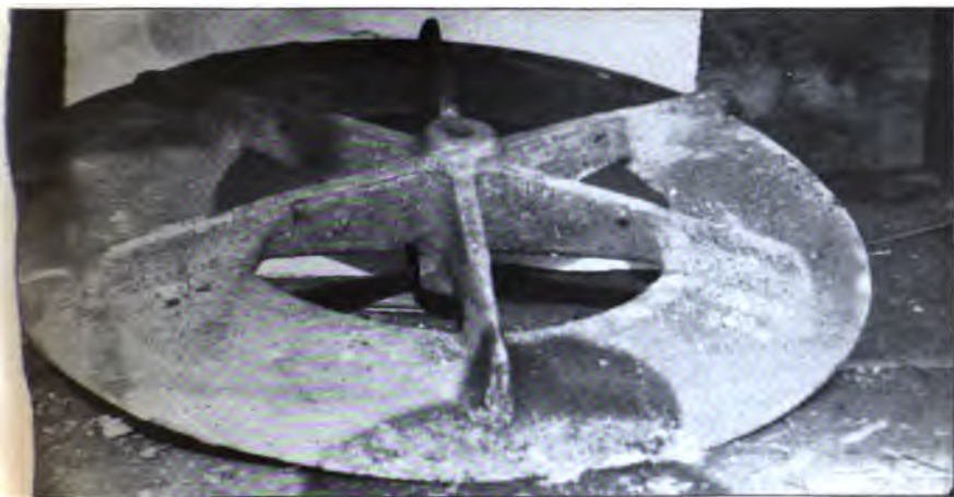
A. DEPOSITING SURFACE FOR CARBON IN ROTATING-DISK PROCESS.
