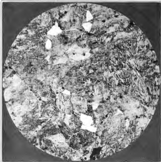
A. HEAT 1347, INGOT A, BUTT, CHROMIUM-CERIUM STEEL HNO 3 ETCH, SHOWING GLOBULAR INCLUSIONS MOSTLY AT GRAIN BOUNDARIES, BUT NO DEFINITE CRACKS. MAGNIFICATION 100 DIAMETERS.
