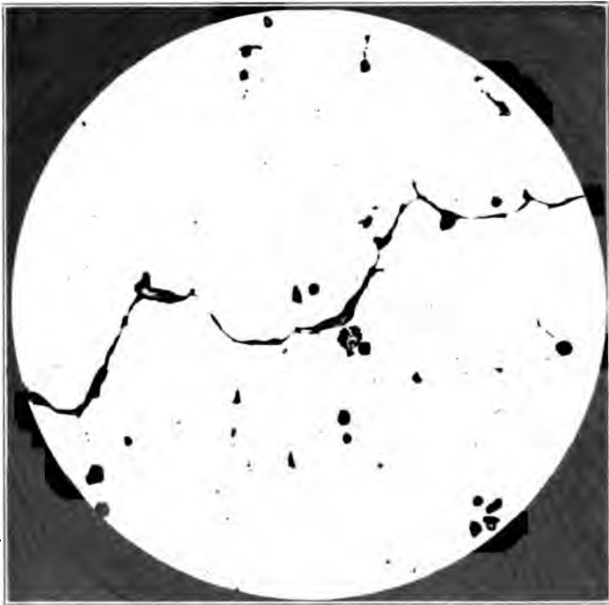
A. HEAT 1363, TOP OF INGOT, CHROMIUM-CERIUM STEEL, UNETCHED, SHOWING CRACKS. MAGNIFICATION 100 DIAMETERS.
