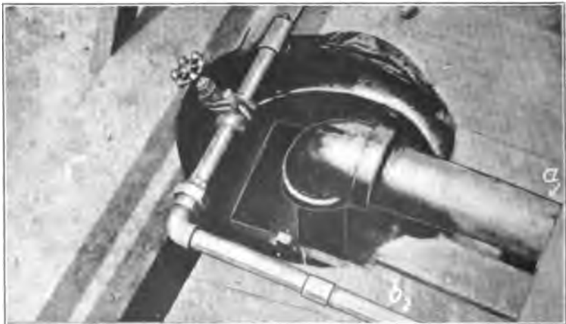
B. OIL ENTERING SECOND STAGE OF DEHYDRATION: a, OIL INLET; b, STEAM INLET.
