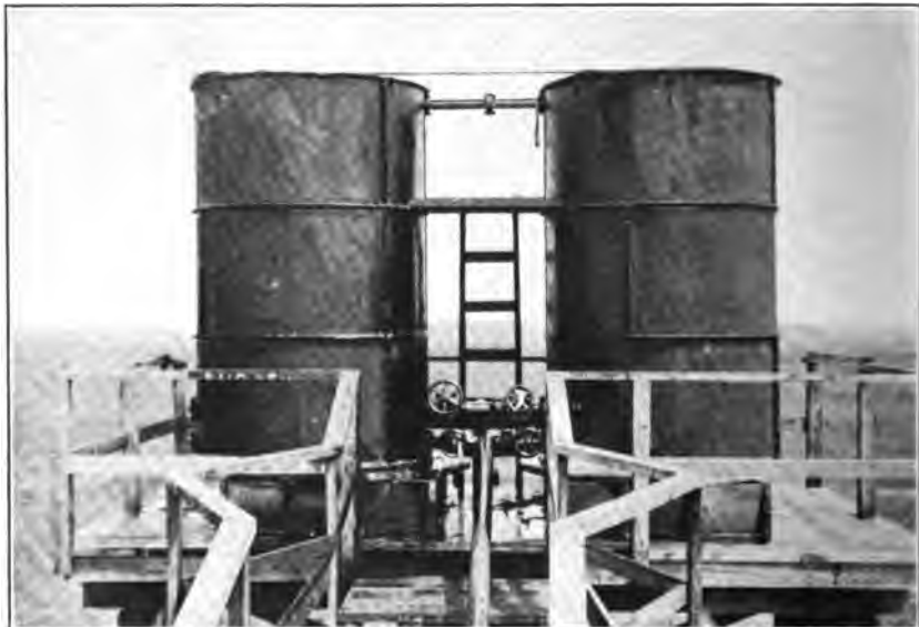
A. TANKS USED FOR MEASURING THE VOLUME ENTERING DEHYDRATION PLANT DURING TEST.
