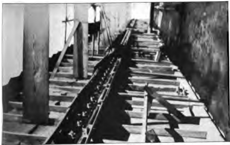
B. GEAR-ACTUATING CYLINDERS IN THE ROLLER PROCESS.
