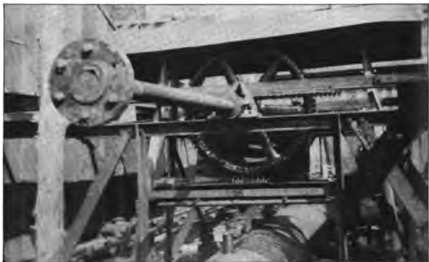
A. DRIVING WORM GEAR, CHANNEL PROCESS.
