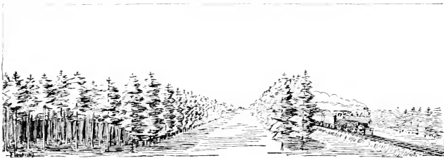
FIG. 83.—A fire line along a railroad with two cleared spaces separated by a double row of trees intended to catch the sparks.
