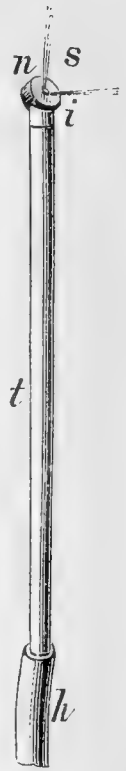
FIG. 5. — Metallic hand pipe with diagonal nozzle; hose, h ; metallic pipe, t ; diagonal eddy-chamber nozzle, n ; its removable face, i ; spray, s .
