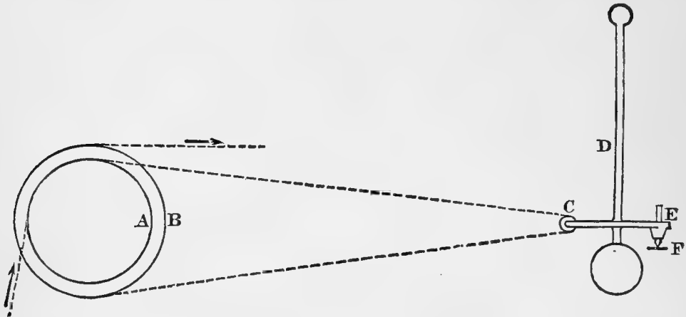
FIG. 2.—The principle of the serigraph.
