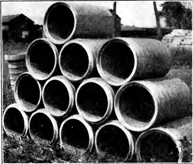
Irrigation pipe with tongue and groove joint.
