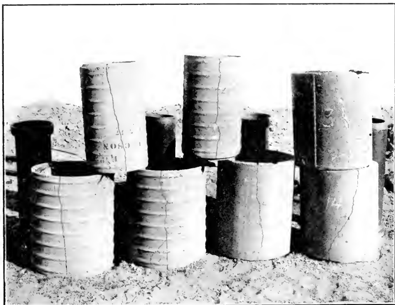
Fig. 25.—Test specimens broken in internal-pressure testing machine.
