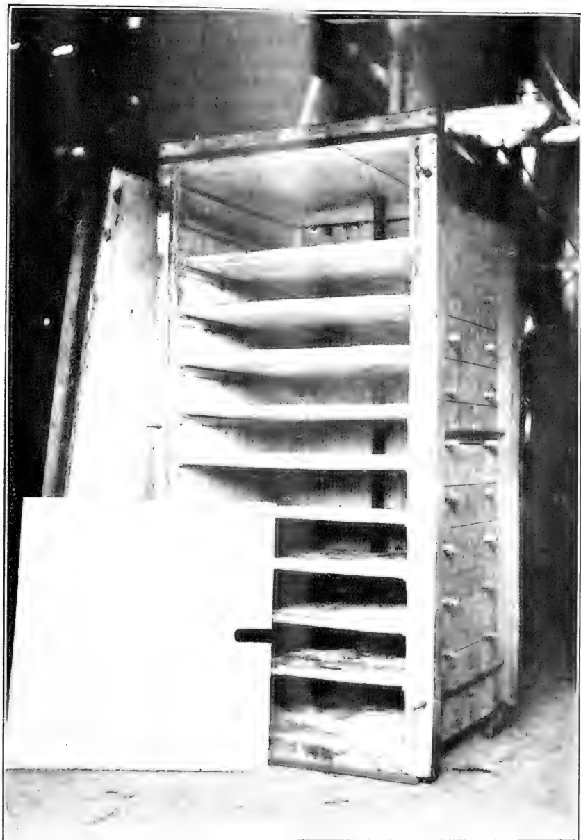
FIG. 2.—Cabinet used for breeding the Muscardine fungus in the Mulgrave Central Mill, Gordonvale. The heavy door stands at the left, and one of the corrugated iron shelves in the foreground. The twenty small tubes through which the cabinet is inoculated are shown on the right side.
