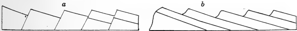
Fig. 1 Diagram illustrating the detailed structure of parts of Becraft mountain: a , as interpreted by Mather; b , as actually existing.
