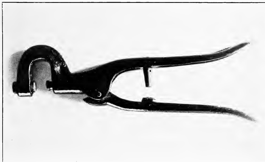
FIG. 2.—Pliers used in attaching the marking buttons.
