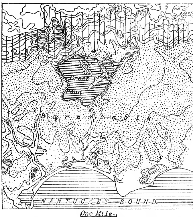
FIG. 4. A portion of the Barnstable atlas sheet, showing the morainial wall on the north and the wash-plain on the south enclosing Great Pond. Deposits of earlier drift form knolls and hummocks along the south shore. Contour interval, 20 feet (from U. S. Geol. Survey).
