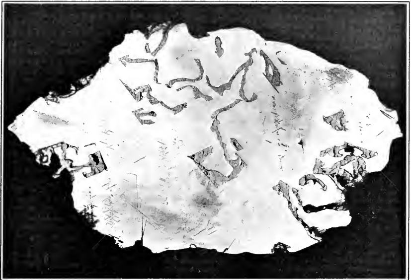
(1). WIDMANSTÄTTEN FIGURES, ENLARGED; (2). SCHREIBERSITE IN ARISPE AND (LOWER) IN TOMBIGBEE IRONS
