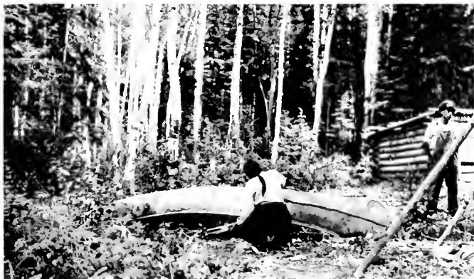
Pitch being applied to seams.
