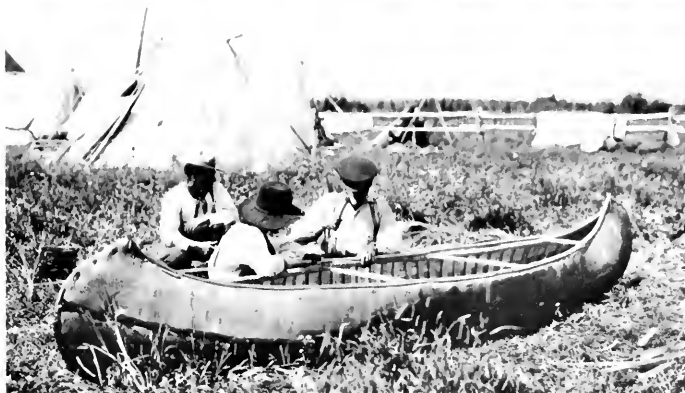
Fitting gunwale caps on new canoe.
