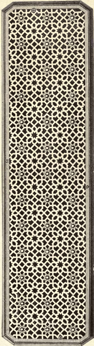
FULL SIZE CROSS SECTION OF BUNDY RADIATOR LOOP.
