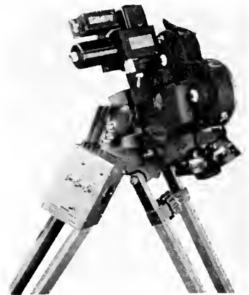
New two-speed stop-motion motor shown mounted on Arriflex camera.
