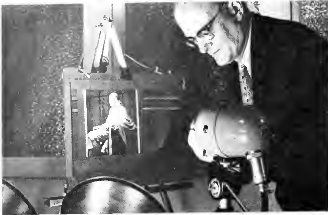
Adjusting television camera for transmission of still picture over standard telephone cable is Bell engineer, C. Raymond Kraus.
