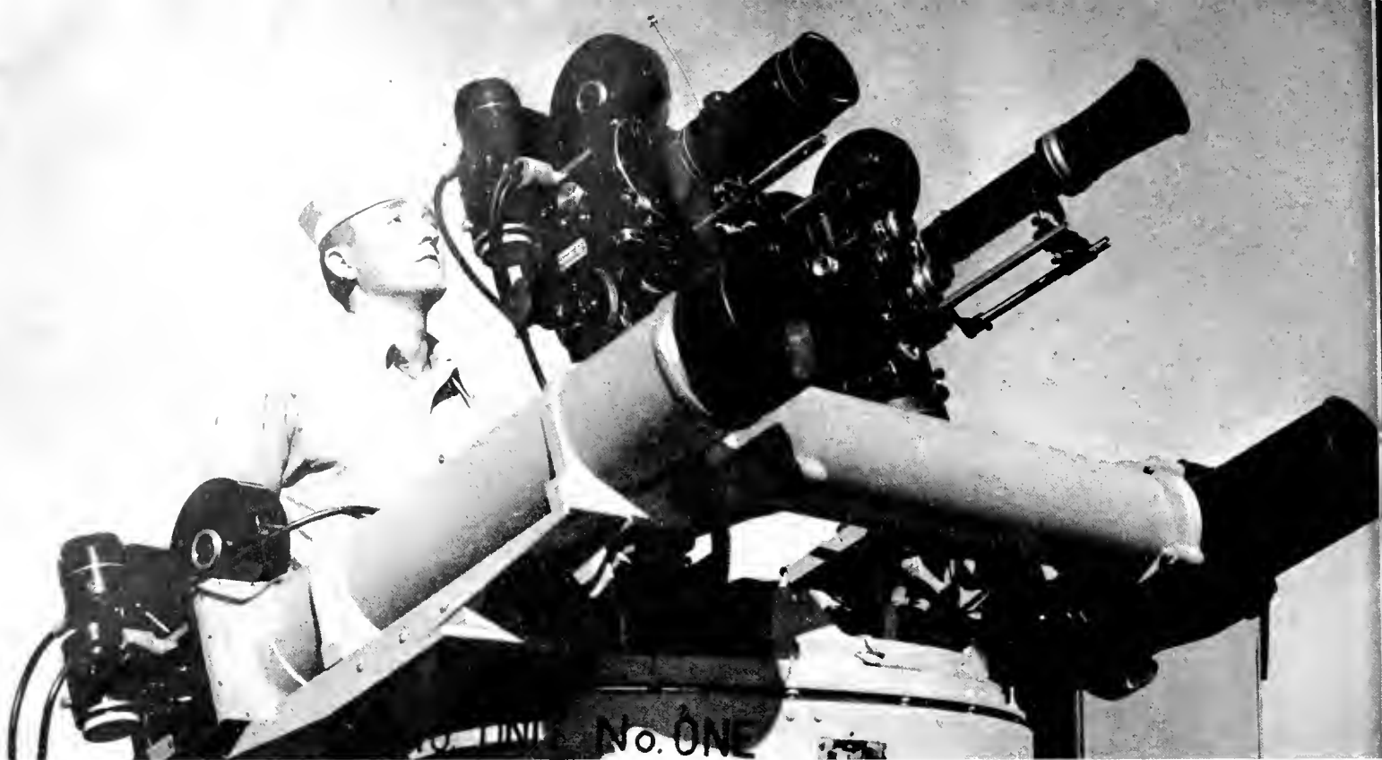
Multiple Mitchell Cameras on Mobile Turret of U. S. Naval Air Missile Test Center, Point Mugu, Calif. Seventeen 35mm and five 16mm Mitchells are used here.
