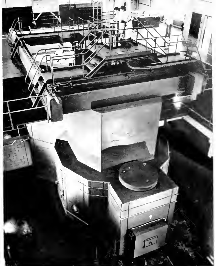
Above: pictured in the Atom Comes to Town is this one million-watt nuclear reactor at the Battelle Institute, helping to develop atomic energy.
