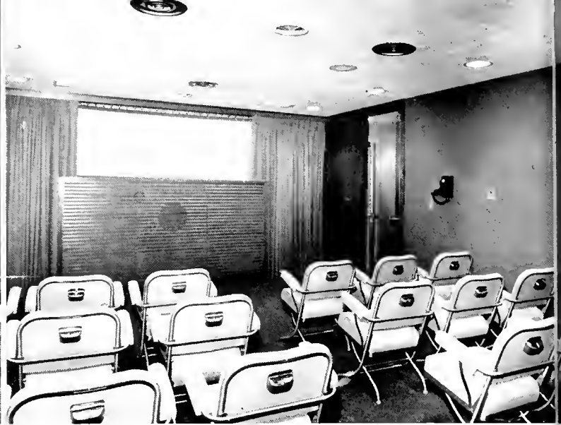
Preview room screen is Vicia Lite 108" wide angle with 8" curvature. In addition to three ceiling speakers, film sound is delivered by a 15" coaxial speaker within front baffle. Mayfair folding chairs have built-in ashtrays; Naughahyde covers; gold bonderized aluminum arms.
