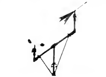
Wind direction is where it comes from. Speed is measured accurately by whirling cups called anemometer.
