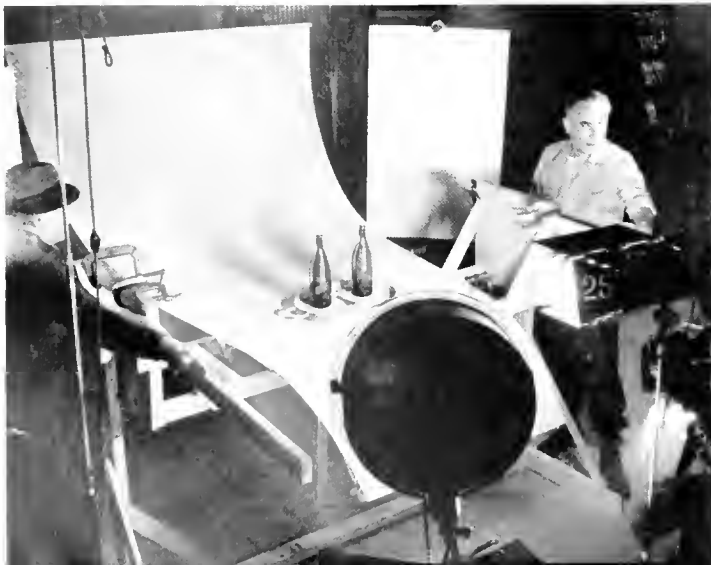
A movable cyclorama rig that helped to eliminate camera moves.
