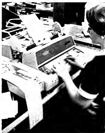
As the Flexowriter prints the order from pre-punched customer cards, a paper tape (foreground) is punched. This combines all fixed and variable data needed for the big computer.
