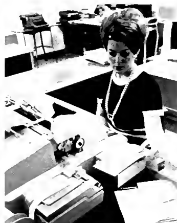
Repetitive information, such as customer name and address, are entered from pre-punched master cards. Variables, such as film show date, are then entered from the keyboard.
