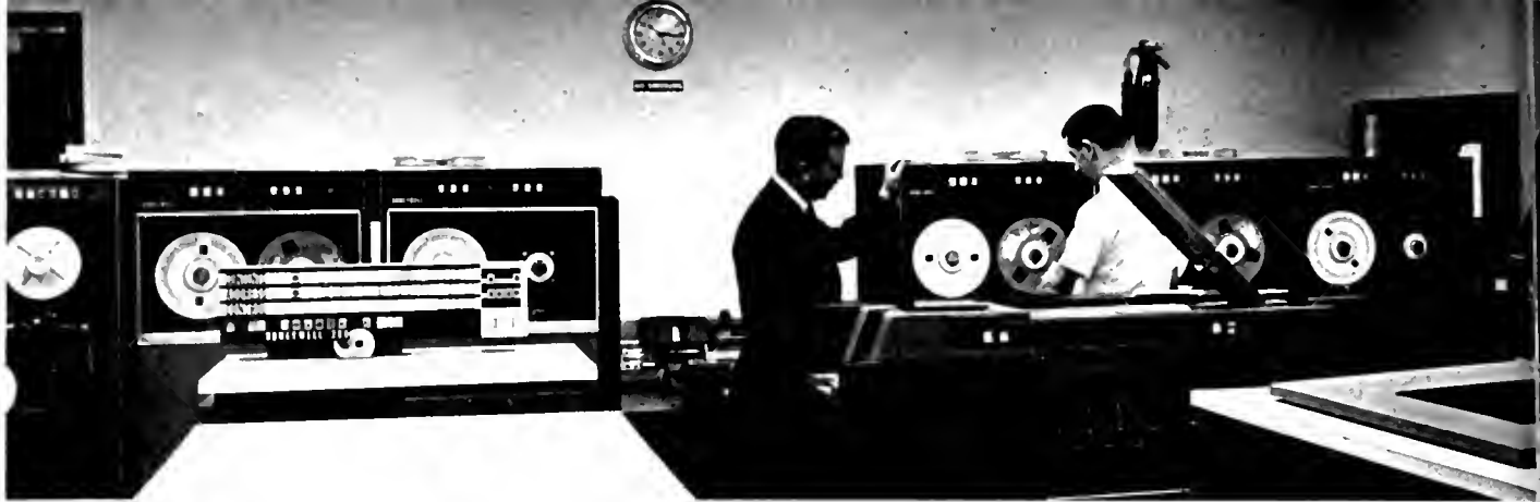
Heart of Modern's EDP system is a Honeywell 200 computer with its five magnetic tape drives, tape reader, 600 lpm printer and 16K main memo-
