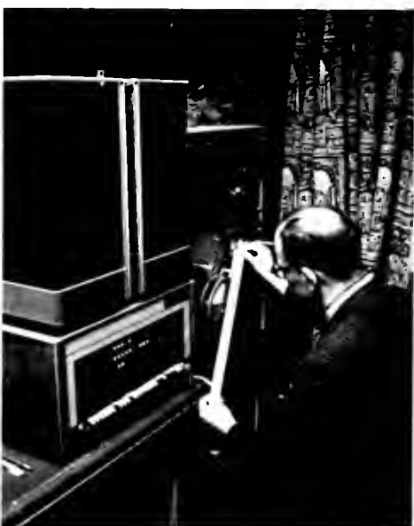
Computer is on the left; automatic tape punch is at right. Director is shown removing a piece of punched tape from rack, ready for the stand.
