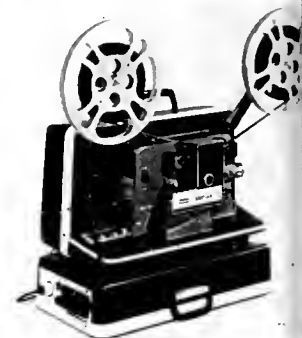
Graflex 16 Arc Light Projector uses the new G-E "Marc 300" quartz arc lamp and a power supply unit to pour brilliant light onto screens. Other features: transistor amplifier; twin 5" oval permanent magnet speakers; fumble-free film loading; pushbutton, color-coded operating controls; an adjustable film gate; and single-lever reverse operation. Weight 37 lbs.; power supply weighs 26 lbs. Write Graflex, Inc. (see page 64) for technical literature and dealer sources.
