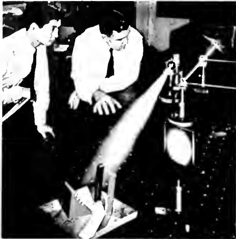
Hologram is made by using laser beams to illuminate both subject and reference source. Scenes were shown to editors during Mr. Hunt's address.
