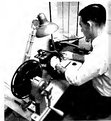
Hot splicing is done on Bell & Howell equipment like this "foot splicer" pictured in scene above.
