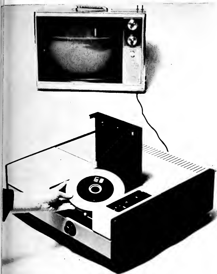
TOP — The EVR player is readily connected to any conventional TV receiver with a single wire.
