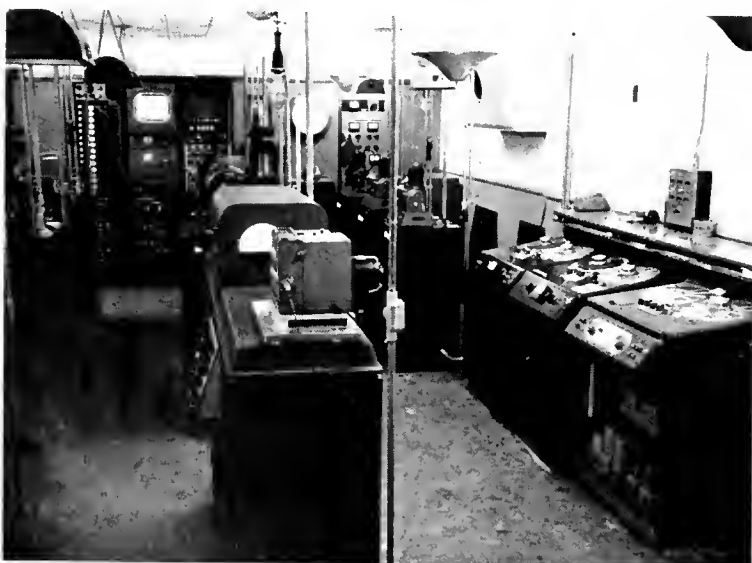
Up-to-date kinescope operation, with recording unit in center, at CBS-TV studios in Hollywood. The network used this TV recording set-up in the early 1950's. (Reprinted by permission of the Regents of the University of California.)
