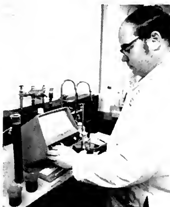
Above: lab's chemist is using his pH meter to test acidity and alkalinity of solutions. At the right: analysing the developing solutions ("titrating") is another necessary procedure to safeguard the processing results.
