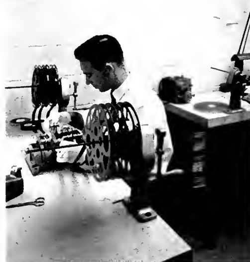
Preparation of film for processing: conforming of original A & B rolls to cut the work print.
