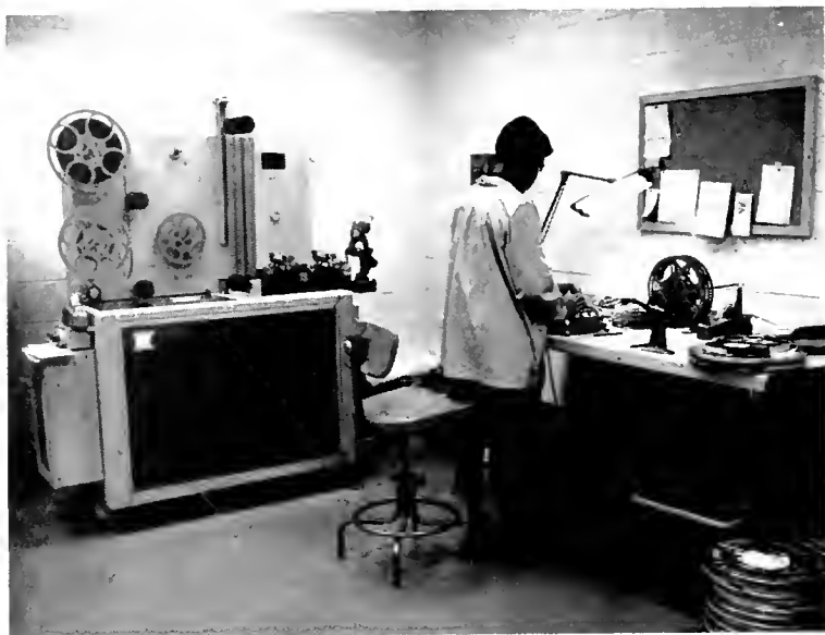
Magnetic striping of sound on film is done on the Reeves sound striping equipment pictured at left in scene above; Byron pioneered in this field.
