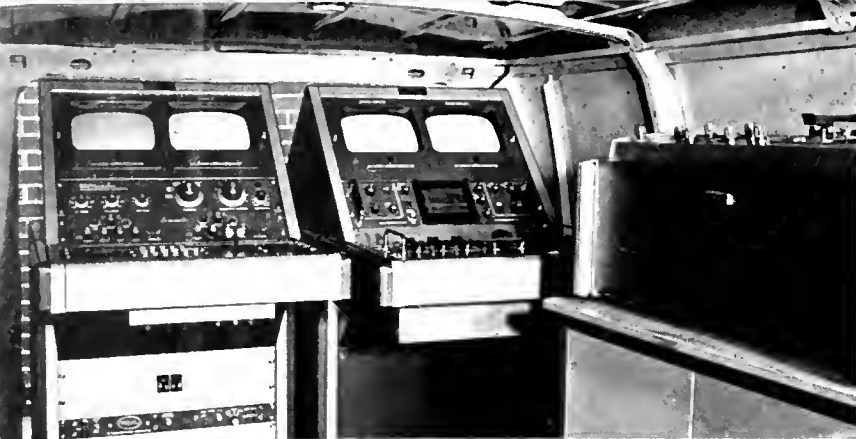
The videotape recording training gear is contained in small mobile van (right). Standard production system shown inside includes power supplies, editing equipment and videotape recorder.
