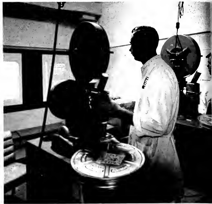
These high-speed print inspection projectors, manufactured by the Hollywood Film Company, help to assure the ultimate quality of all prints out of the laboratory. This final phase of the processing procedure is the "proof of the pudding" from the customer's viewpoint . . . and at point rigid quality standards must be met or prints are rejected.
