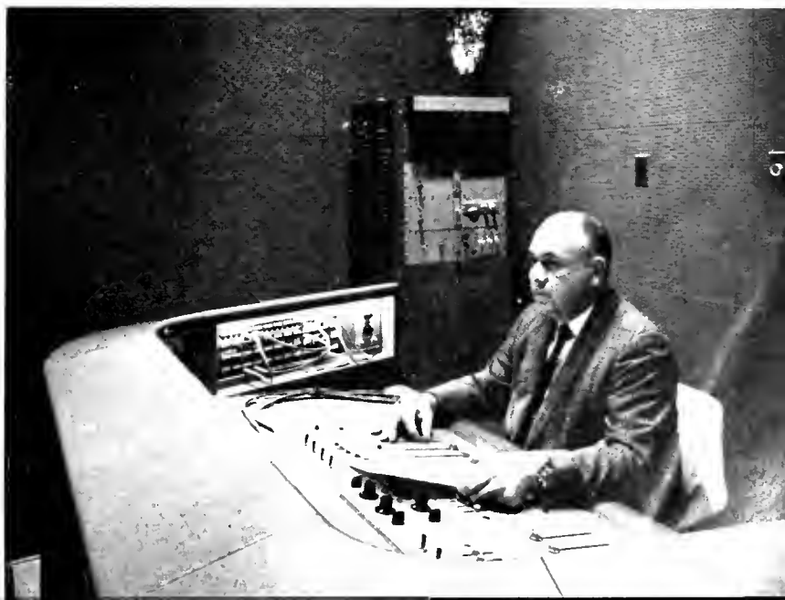
This 16/35mm projection room opens into both narration studios, sound mixing studio and the theater. Projectors are Bell & Howell 16's and Century and Simplex 35's, with Westrex motor drives, RCA Selsyns for interlocks; 35's also have Xenon light source. Below: Richard "Pat" Patton, manager, Sound Department, is behind the Westrex sound mixing console.
