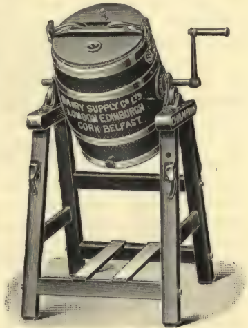
SMALL HAND-POWER END-OVER-END BUTTER CHURN
