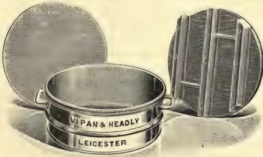
LEICESTER CHEESE MOULD WITH TIN (LEFT) AND WOOD (RIGHT) FOLLOWERS
