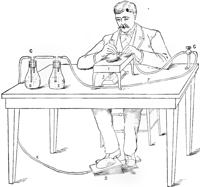
FIG. 61.—Apparatus for inflating larvæ: B , foot-bellows; K , rubber tube; C , flask; D , anhydrous sulphuric acid; E , overflow-flask; F , rubber tube from flask; G , standard with cock to regulate flow of air; H , glass tube with larva upon it; I , copper drying-plate; J , spirit-lamp.
