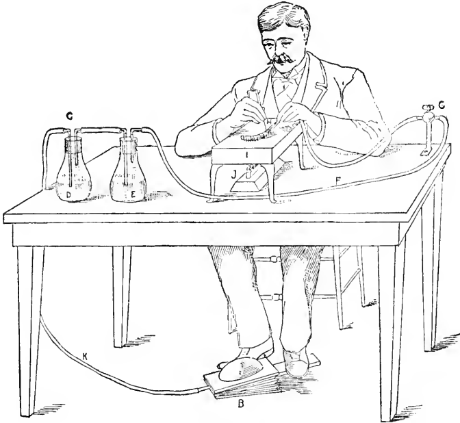
FIG. 61.—Apparatus for inflating larvæ: B , foot-bellows; K , rubber tube; C , flask; D , anhydrous sulphuric acid; E , overflow-flask; F , rubber tube from flask; G , standard with cock to regulate flow of air; H , glass tube with larva upon it; I , copper drying-plate; J , spirit-lamp.
