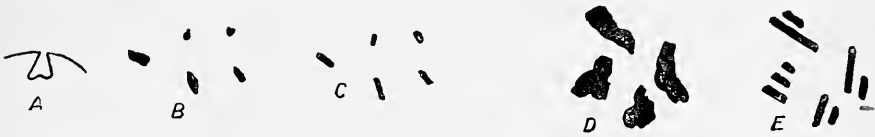
Fig. 167.—A, Opening for wire; B, small holes; C, small holes plugged; D, large defects; E, large defects plugged.
