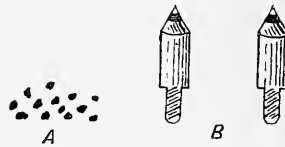
Fig. 105.—A, Diamond chips; B, diamond chips set into holders and ground to a point.
