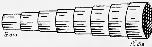
Fig. 221.—Pivot Gauge. Half size.
