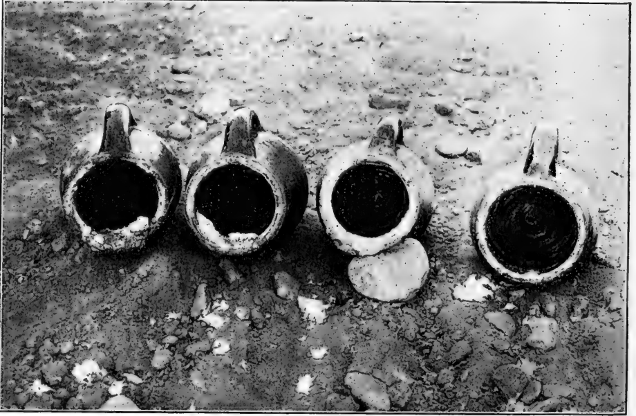
FIG. 52.—Acid generators showing residue remaining because of careless emptying. (After Pierce, P. C. Jr. Ent.)
