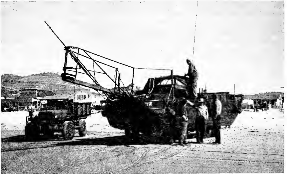
FIGURE 78. DUKW showing pulpit and spear ready for use. Truck is sometimes used for pulling the carcass to the beach. Photo by John F. Janssen, Jr.
