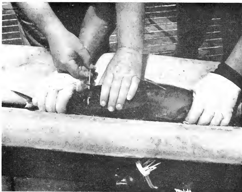
FIGURE 11. Inserting a Type F tag on a small yellowfin tuna. The tag insertion needle shown is too long when used on small fish, because the needle rides into the side of the cradle. The tag insertion needles have since been made shorter. Photograph by C. E. Blunt, Jr., May, 1953.
