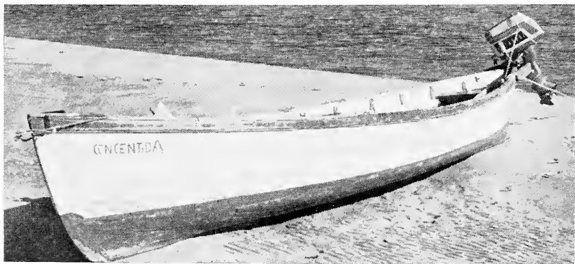
FIGURE 3. A typical open boat, approximately 18 feet long, used in the central Baja California sea turtle fishery. Photograph by the author, February 1962.
