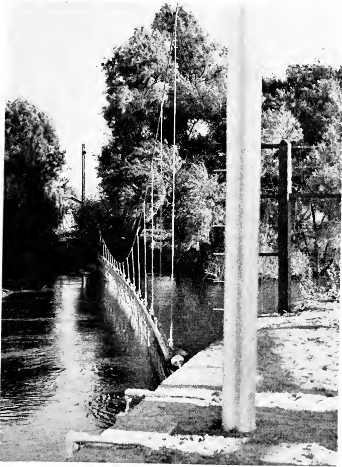
Figure 11. Experimental electric fish screen now being tested near Mendota. Photograph courtesy of Henry T. Bucky
