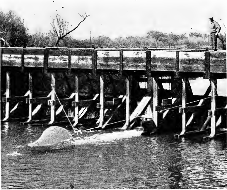
Figure 10. Fyke net being used to estimate the loss of baby salmon into a canal. The canal was taking very little water when this photograph was made and practically the entire flow was going into the fyke net. Photograph by Donald H. Fry, Jr.
