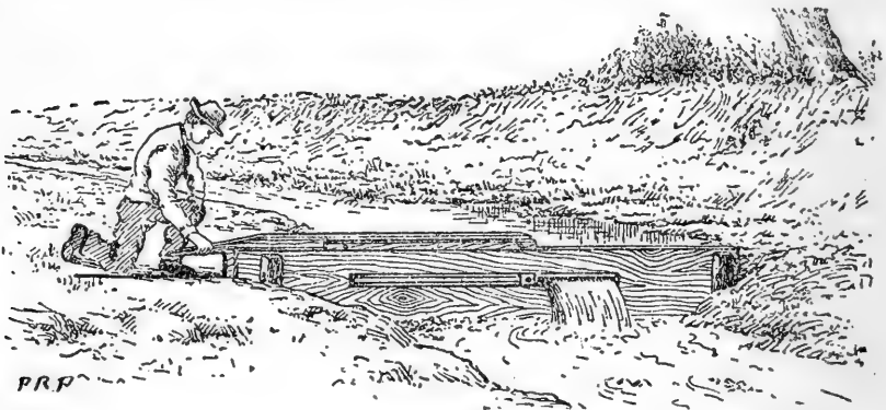
Measuring miner's inches in a small stream or ditch.
