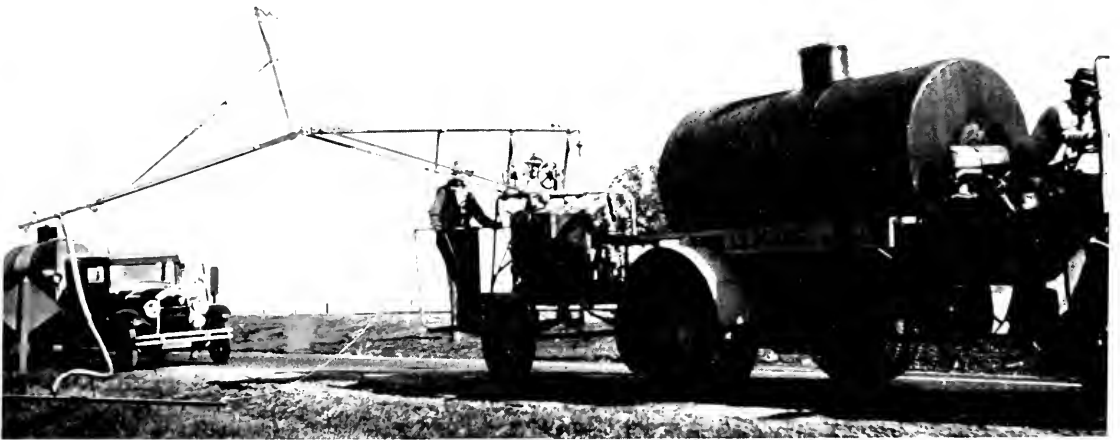
THE TANK CORPS with numerous units equipped like the above is engaged in the annual preliminary skirmish against old Demon Fire Hazard on all State highways. A weed spraying outrigger on an oil spreading trailer makes combustion sure and complete with a liberal dosage of inflammable mixture.
