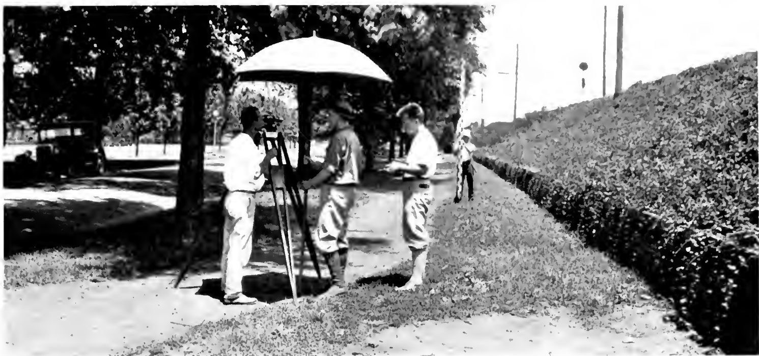
GEODETTIC SURVEY LEVELING PARTY. The umbrella is to protect the instrument, not the observer.
