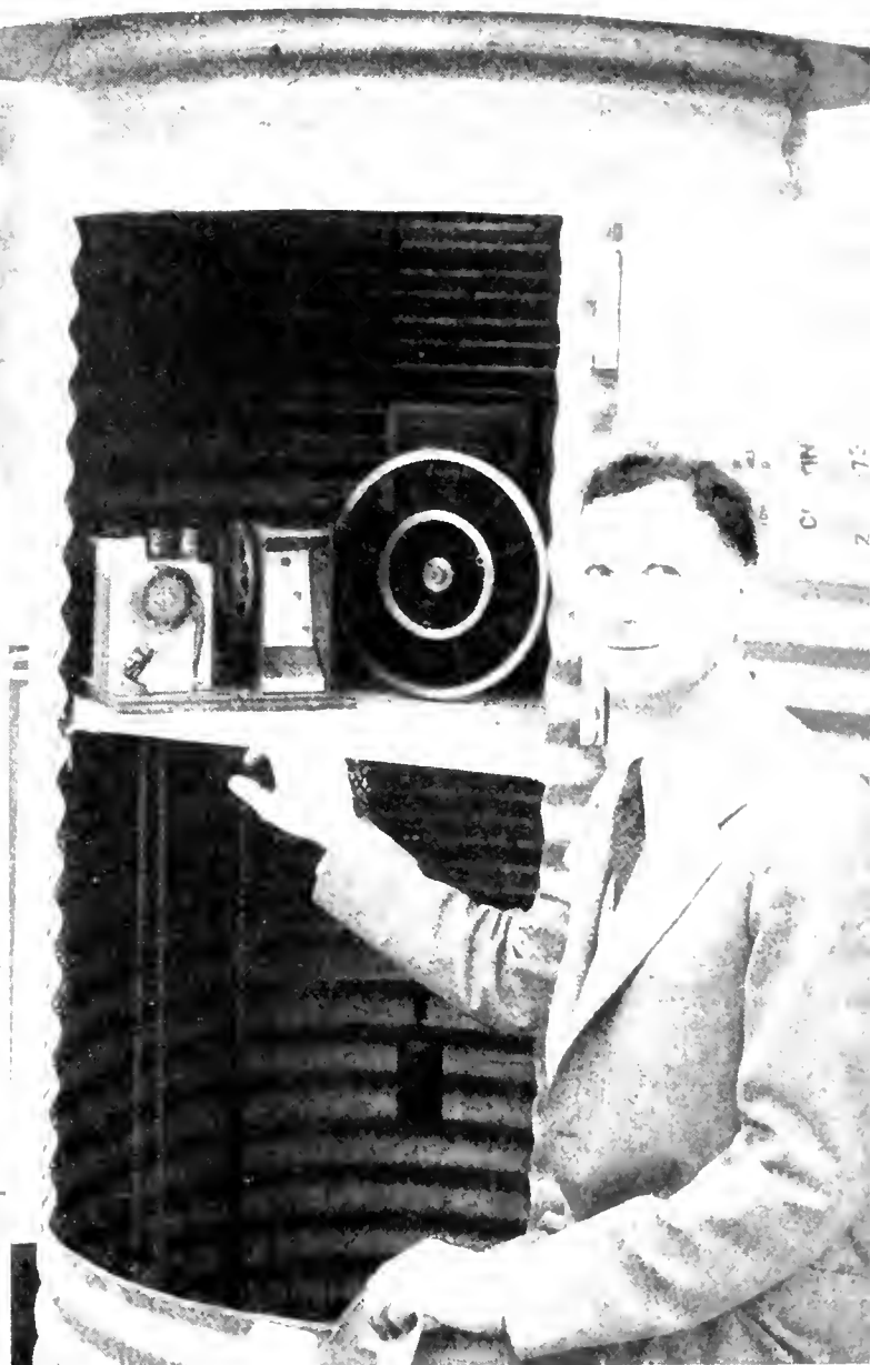
ON GUARD in little shelter houses along 13 California streams is this Ingerson automatic radio stream gage signal apparatus that sends out warnings of flood dangers. Front and rear views of the gage keying device and transmitter are shown in pictures 1 and 2 and inventor Irvin M. Ingerson, associated hydraulic engineer of the Division of Water Resources is shown with the installation in No. 4.
