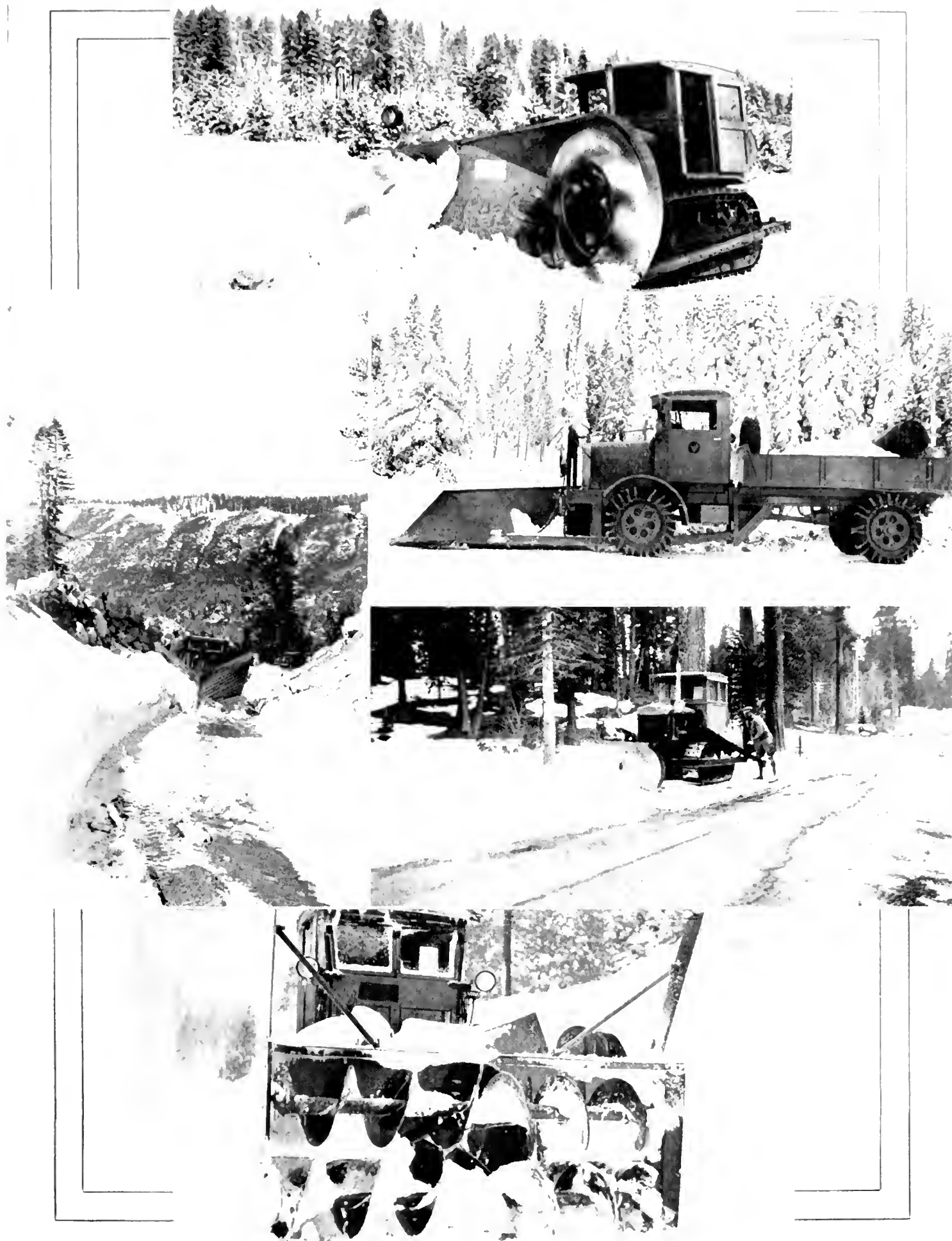
SNOW REMOVAL EQUIPMENT keeping California State highways open this winter numbers 168 units of various types some of which are pictured above. At top, a tractor type rotary, the business end consisting of a V-plow with a rotary on each side. Below, right, are speed type and tractor push plows. At left, a large V-type push plow and at bottom an auger blower type rotary.
