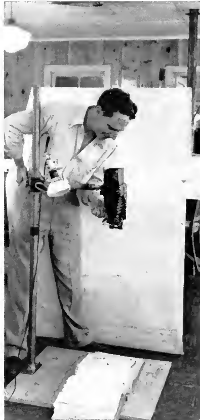
Left—Eastman 9x12 cm. Recomar camera and accessories set up for photographing records. Note scotch tape marking position of books to be photographed. Photos were taken at 1/50 sec. at f-11 on super XX film using a No. 2 photo flood. Focusing was done with the aid of a ground glass. The above "f" stop gives sufficient depth of focus to cover various book thicknesses. Right—Note ease with which photo may be read with a two power lens. A 5"x7" print can be easily read with the unaided eye
