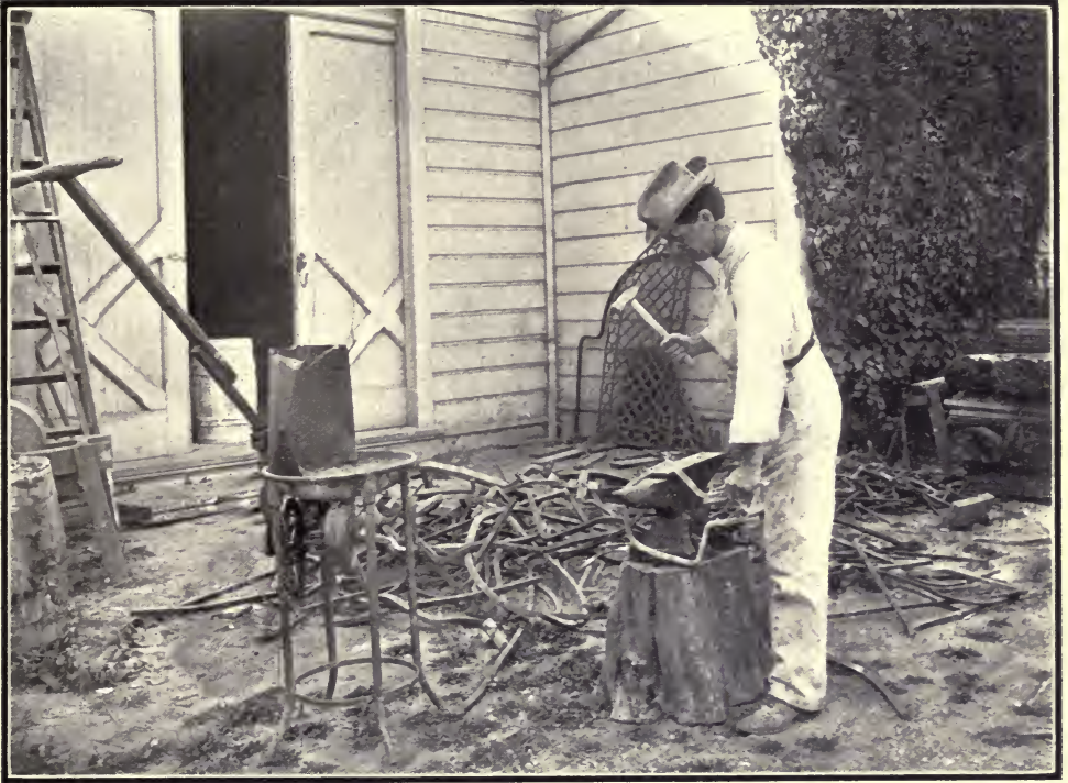
"A sculptor must also be something of a machinist." As the clay in the large statues will not stand alone, the sculptor forges the iron frame-work which outlines the general form around which is moulded the clay.
