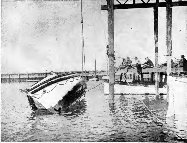
CAPSIZING TEST WITH THIRTY-FOUR FOOT LIFE BOAT.
