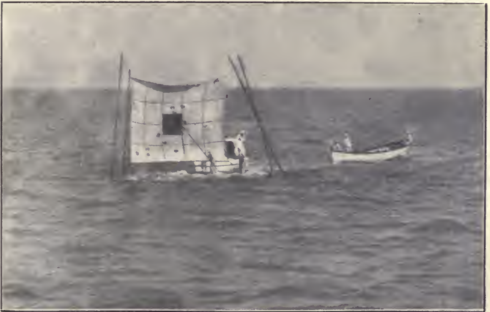
This target is twenty-one by seventeen feet; distance sixteen hundred yards. Speed ten knots. Gun six inch and the number of shots is twelve.
