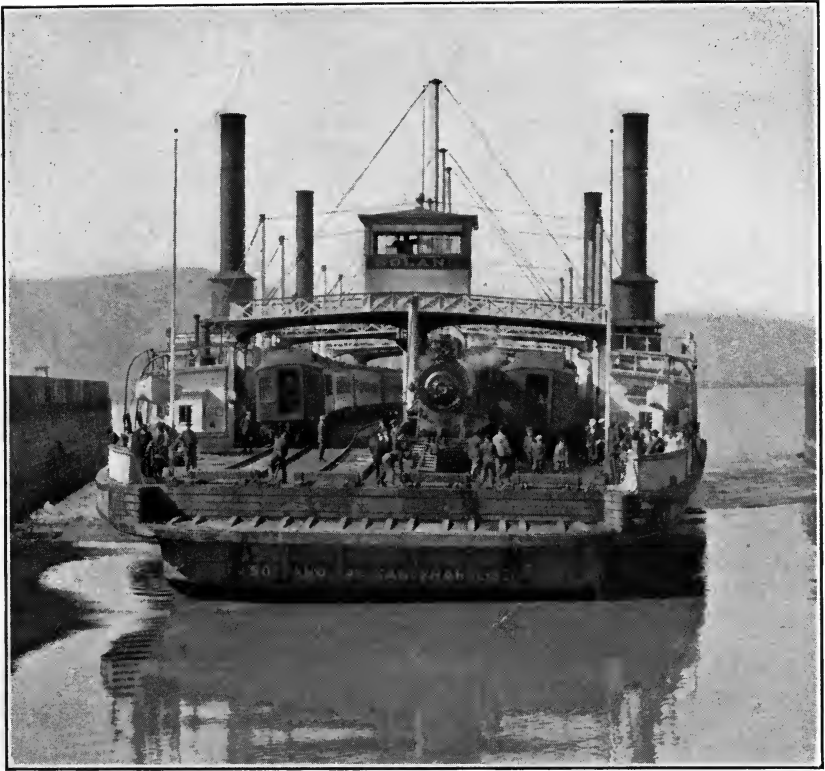
The Solano, the largest ferry boat in the world, used to carry passengers and a train of cars across Carquinez Strait, near San Francisco.
