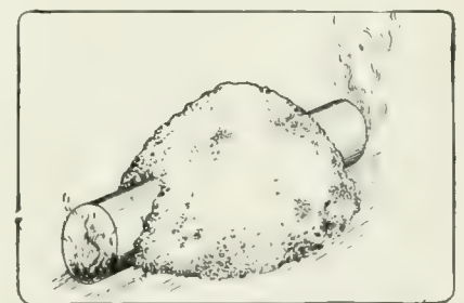
Fig. 3 Showing How Materials may be Heated by Means of a Fire in an Old Stove Pipe
