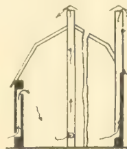
Fig. 1. Two methods of installing ventilating system.
