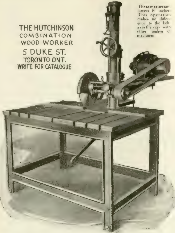
No. 1—Operated by 1½ H. P. motor. Average cost for power in Toronto, $1 per month. Same construction as the No. 1 machine, except that the motor is attached to the two steel rods and slides with the saw.
