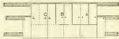
Laying slate in putty.
