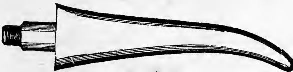
TOOTH OF EYER'S PATENT HARROW. (See p. 474.)
