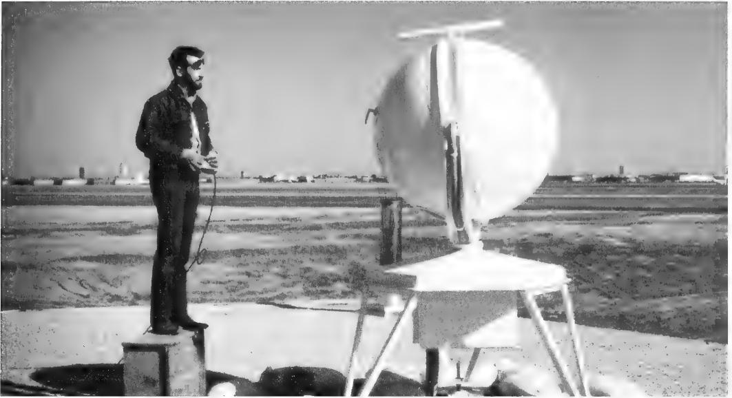
The work of Vic Solman and Hans Blokpoel on how to avoid collisions between birds and aircraft led to innovative uses of equipment. Here summer student Wayne Gemmell aims a radar, usually used to track weather balloons, at a flock of migrating Snow Geese (Photo credit: H. Blokpoel).
