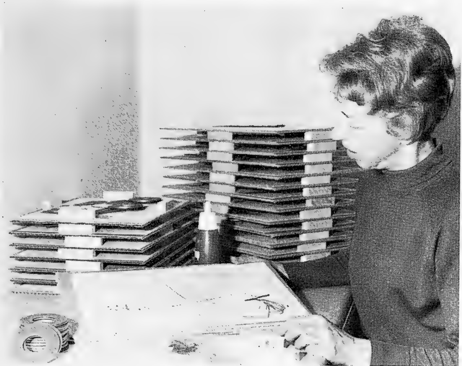
FIGURE V. Photograph illustrating the procedure described for stacking recently mounted specimens supported on corrugates and separated by wood blocks.
