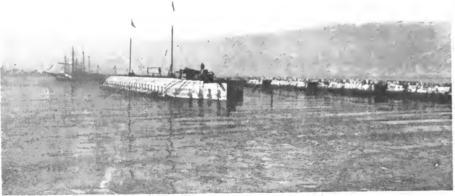
A new timber raft, built by a Canadian at Hommelvik, Norway, 360 feet long, 42 feet beam, 18 feet deep, which outrode a heavy gale in the North Sea. The possibilities of dispensing with ship bottoms in the transport of timber is engaging the attention of Canadian timber exporters.
