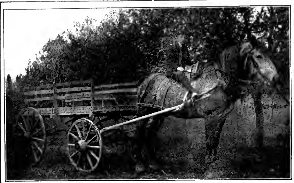
The wagon used in the orchard at La Trappe, Que. Note the strong springs used to protect the fruit from bruises.
