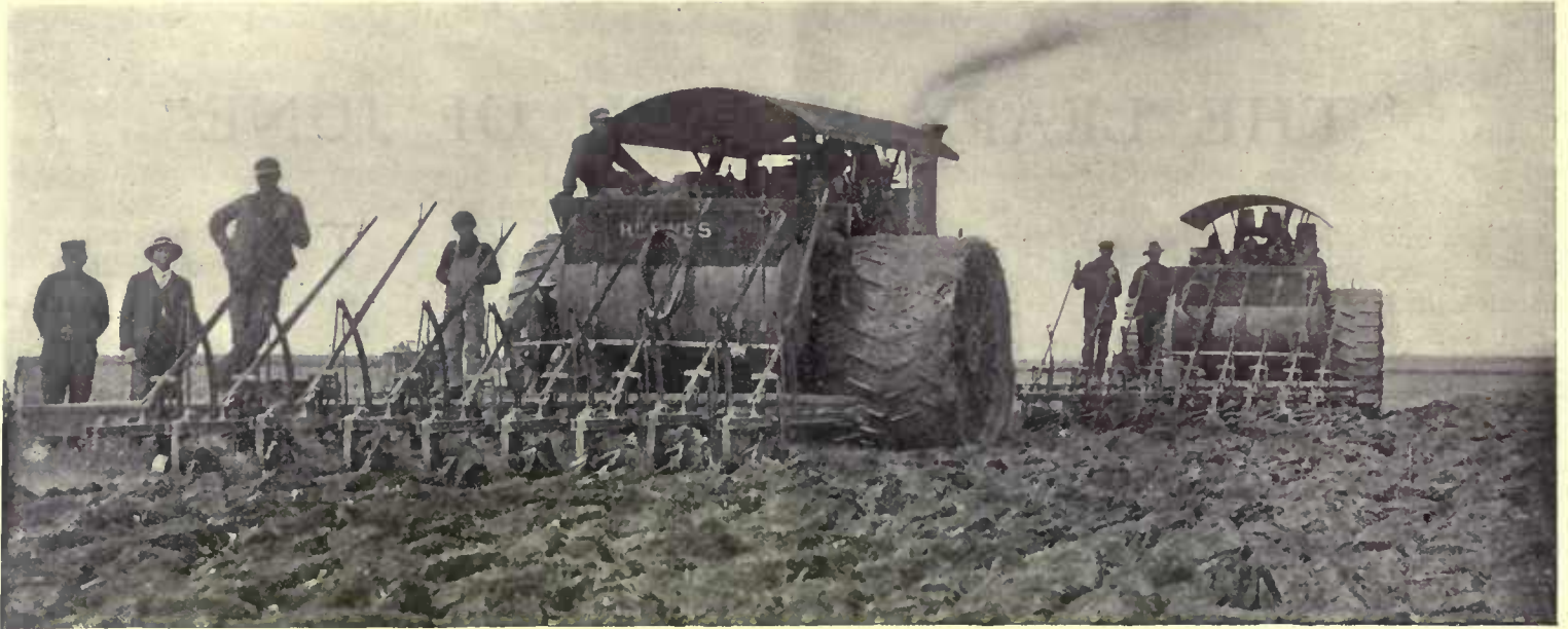
Two steam ploughs breaking up the prairie in the Francis District, Saskatchewan. They belong to Robert Moire and they have ploughed one hundred acres in twenty-four hours.
