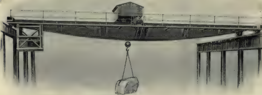
Photo of 5-ton Motor Travelling Crane, 60-foot span
