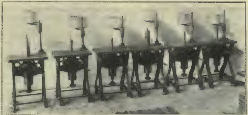
Fig. 5.—Machines Ready for Ramming Cores.
