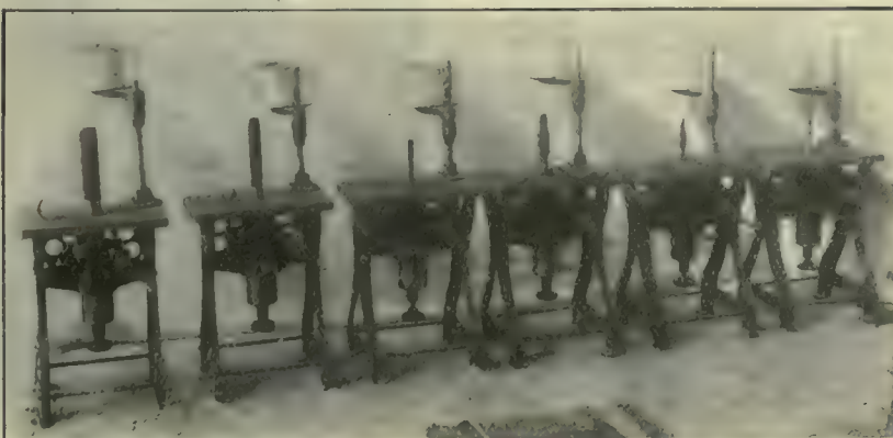
Fig. 4.—Wadsworth Machines After Cores have been Formed.
