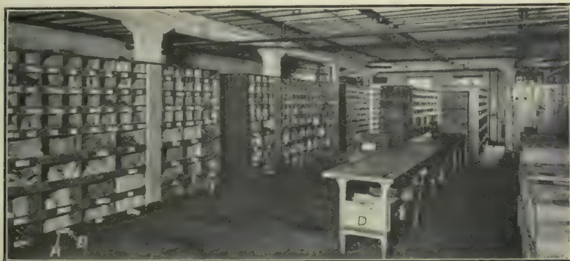
The Stock Room of National Cash Register Co., Toronto. A is the Card giving Name and Number of Part. B is card made in Quadruplicate, One Copy being Sent to Stock Department showing Quantity of Stock Ordered. When it Comes to Hand, it is Checked by Stock Men. C is Signal Bell. D Shows Small Boxes Used for the Easy Handling of Parts.
